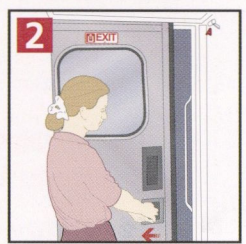
2 Door may be pulled open manually if power fails.
